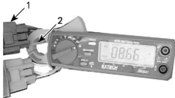
DC CURRENT TEST WITH INDUCTIVE AMMETER
