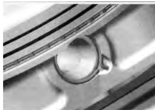
CORRECT POSITION OF THE PISTON CIRCLIP
