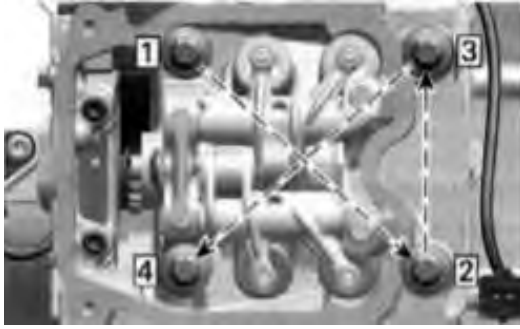
TIGHTENING SEQUENCE-M10 CYLINDER HEAD SCREWS
