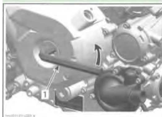
TURN CRANKSHAFT 280° COIUNTERCLOCKWISE
