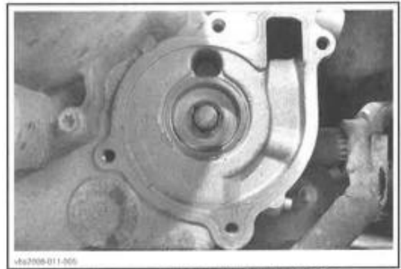
TYPICAL – INNER PARTS OF ROTARY SEAL REMOVED
